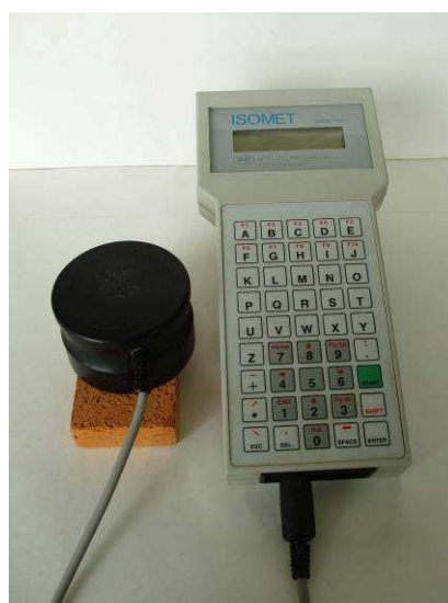
Figure 1.: Determination of thermal conductivity by apparatus IZOMET
